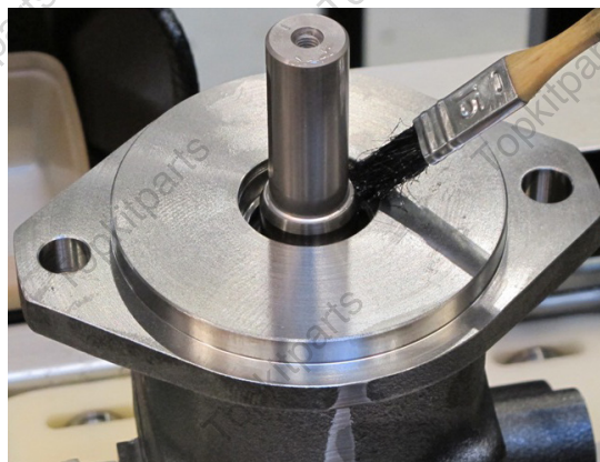
18. Lubricate the sealing surface on the shaft before assembling the shaft seal.
